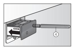
■ Push the module into the slot until it locks into place.
